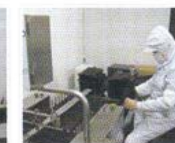
Inserting a tray and a desiccant
